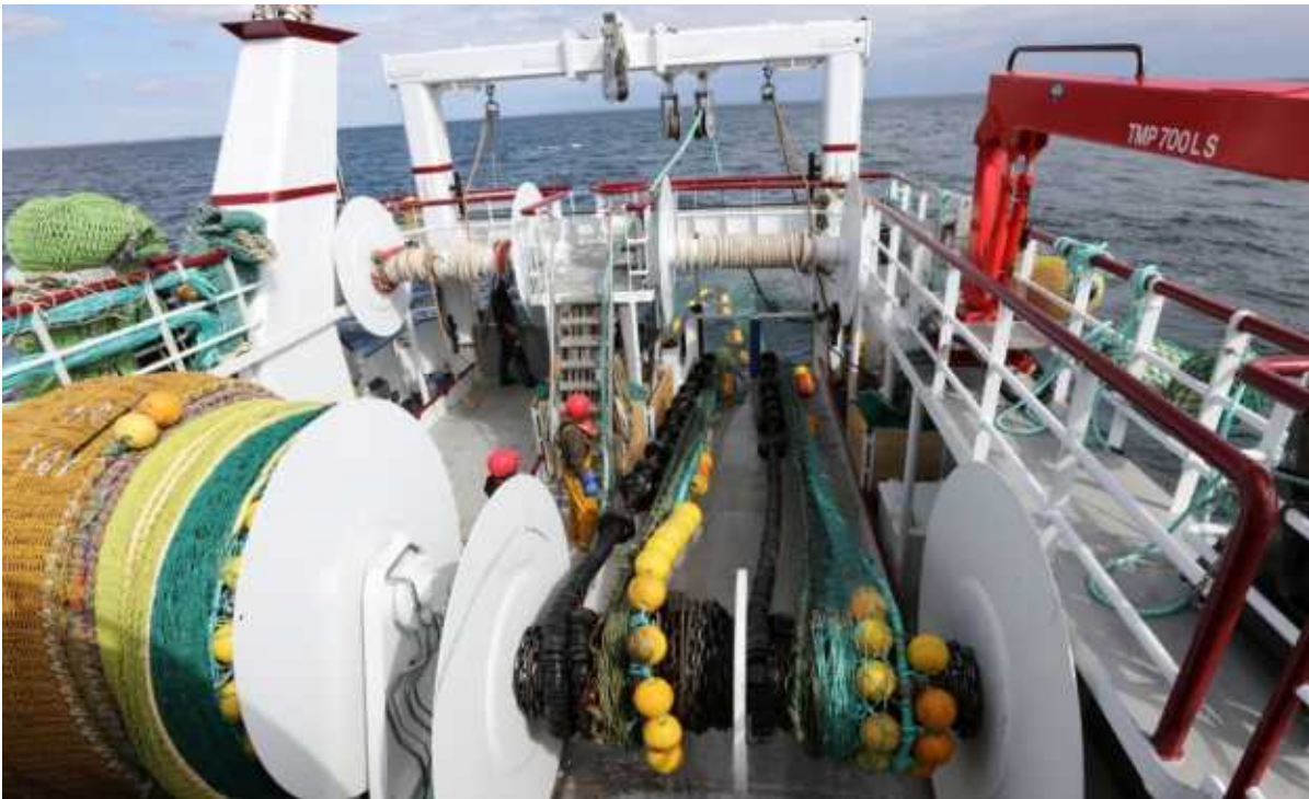
Two net drums are positioned forward of twin bagging drums atop the full-length shelterdeck.
