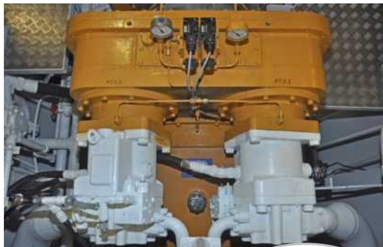
▲ Two hydraulic PTOs are mounted on the Heimdal gearbox.
