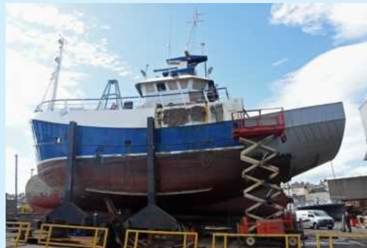
The new transom stern section being welded onto the former Peterhead seine-netter Tranquility at Macduff.
