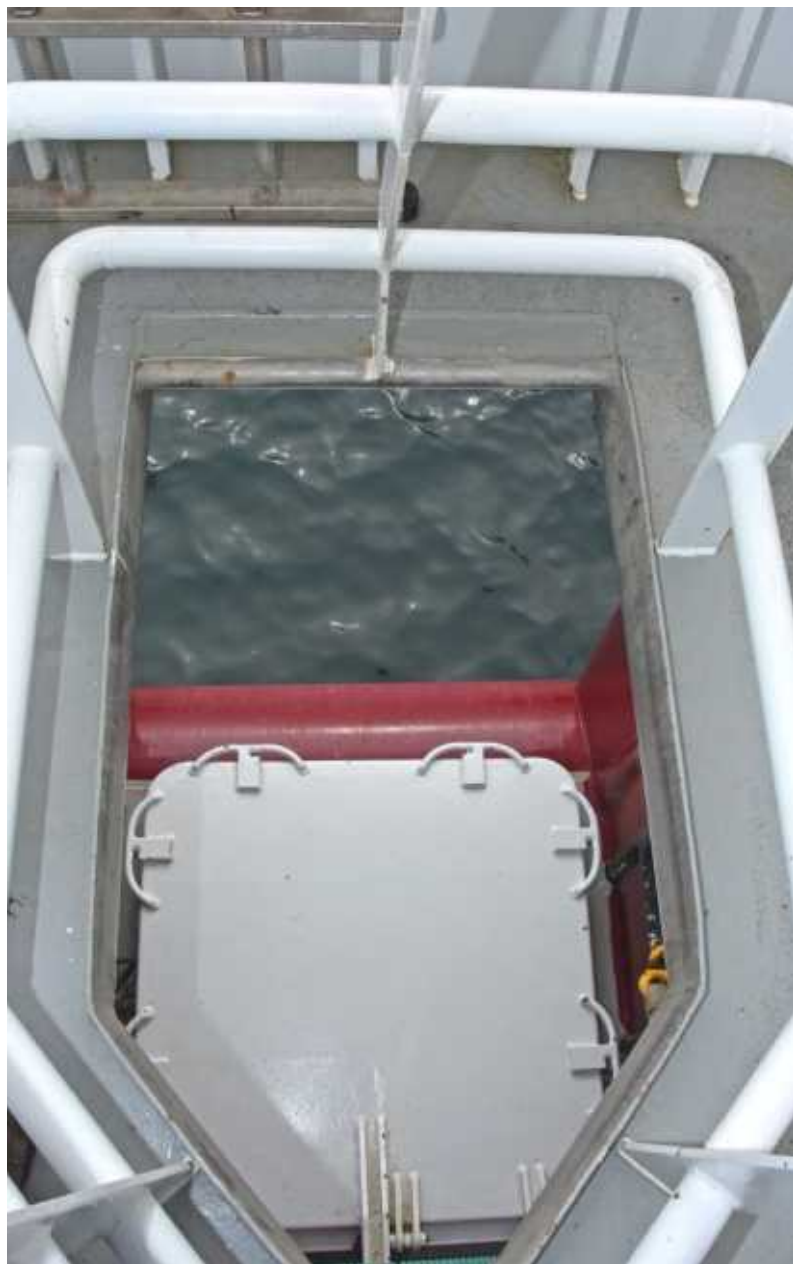
Catches are taken aboard through a centrally positioned opening across the transom above a hydraulically operated and refrigerated reception hopper.
