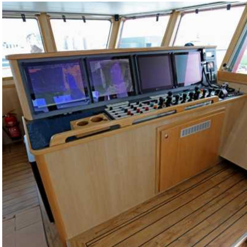
All fishing operations are controlled from the trawl console from which the skipper has a commanding view of gear handling activities and Boy John's movements as starboard boat.
