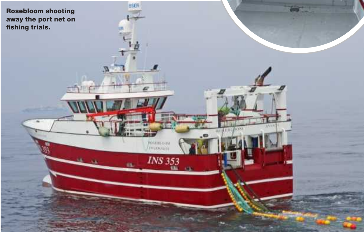
Bagging drums give added flexibility and safety when hauling the high standing pair-seine nets.
