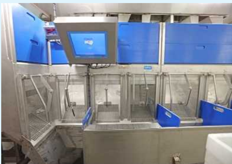
Marel electronic scales and labelling system are located at the starboard side of the fishroom selection hoppers.
