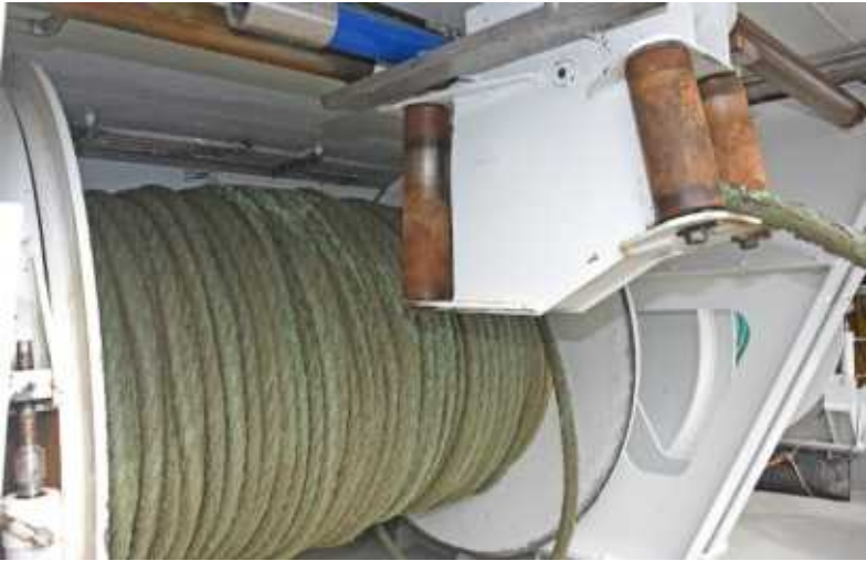
Two 16t power reels manufactured by Kynde & Toft are mounted amidships on the shelterdeck underneath the wheelhouse.
