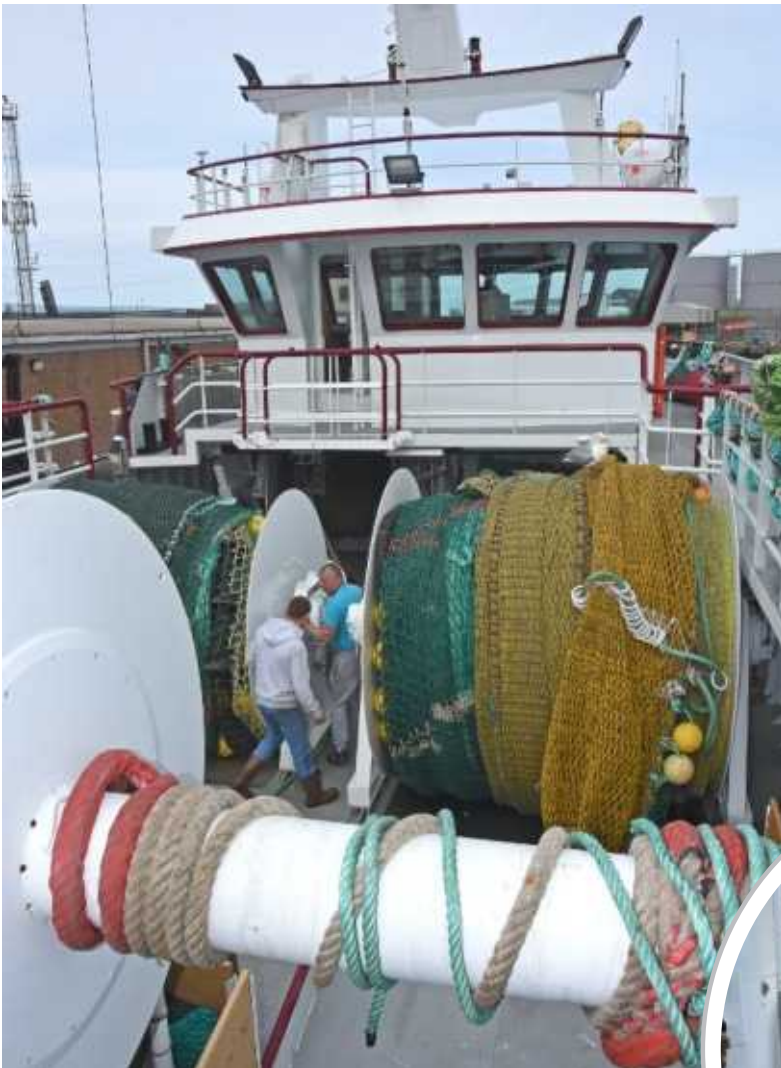
Bagging drums give added flexibility and safety when hauling the high standing pair-seine nets.
