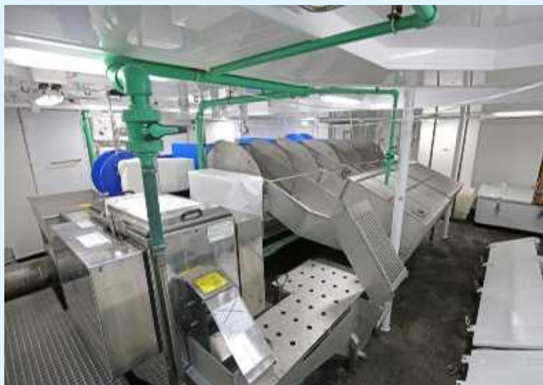
The gutting conveyor and circular selection/washer bins are positioned across the full beam to starboard of the Kronberg MK II gutting machine.
